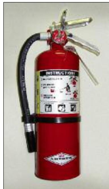
**Be sure to have a fire extinguisher rated for the type of fire at hand: Class A fires are ordinary materials like burning paper, lumber, cardboard and plastics; Class B fires involve flammable or combustible liquids like gasoline and kerosene; Class C fires involve energized electrical equipment such as appliances, switches, panel boxes and power tools. Photograph courtesy of the Fire Safety Council**
